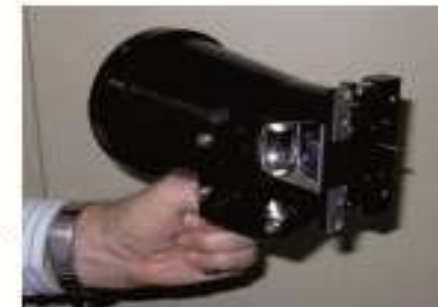
PRISM precursor Dyson spectrometer testbed shows approx. spectrometer size
